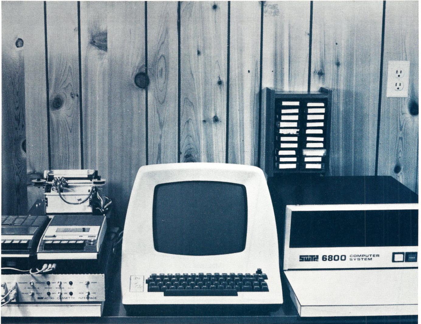
The complete system. MP-68, ADM-3K terminal, AC-30 cassette interface, PR-40 printer, 2 cassette recorders, and a library of tapes.
